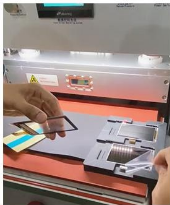
1. Gently peel off the OCA adhesive protective film.
