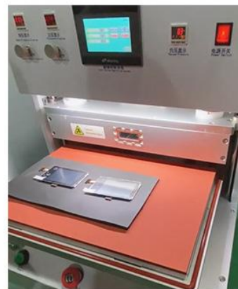
3. Place the aligned components on the bonding platform.
